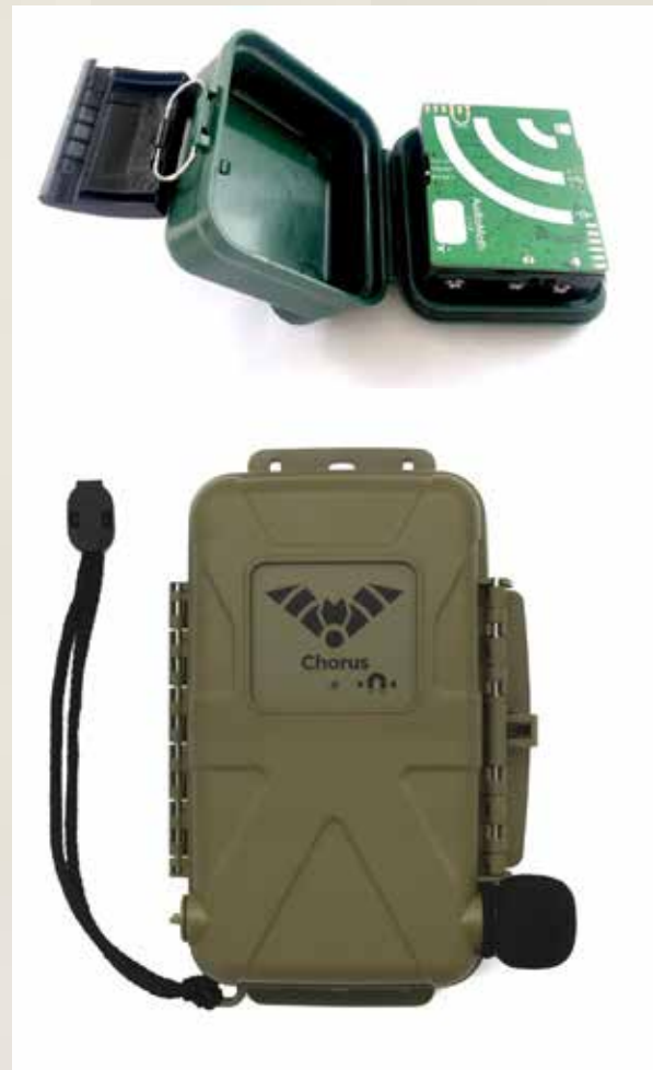
Figure 5. Typical Passive Acoustic Monitors (PAMS) – AudioMoth (top) with waterproof case and Anabat Chorus (below).
