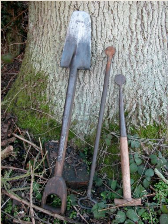
Figure 4. Bark peeling tools.
