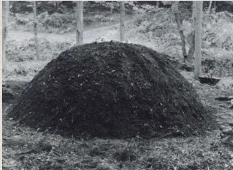
Figure 4 The stack covered and ready for firing
