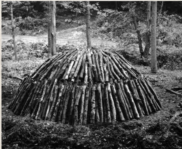
Figure 3 The stack completed and ready for covering
