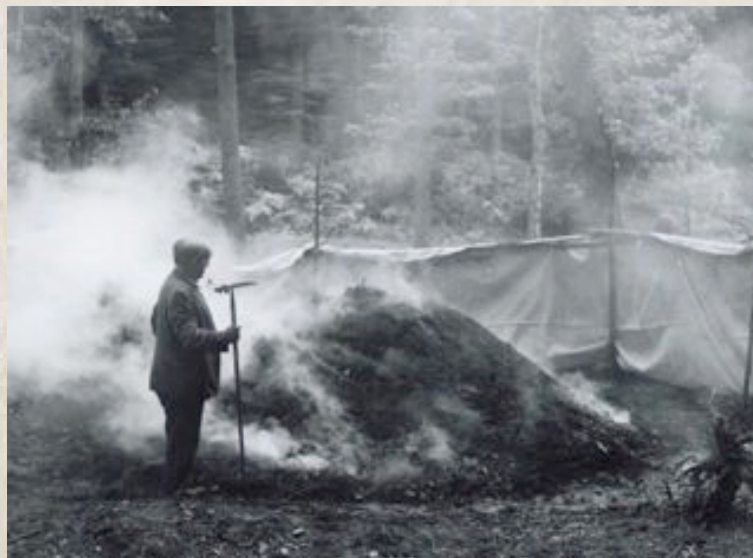
Figure 5 Tending the stack. Screens of hessian shield it from the wind
