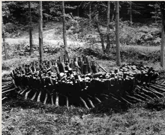
Figure 1 Cordwood assembled prior to raising the stack
